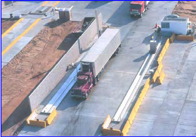
Figure 7-4 VACIS II - Gamma Ray Imaging System
