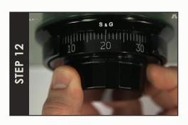
Dial LEFT (counterclockwise) two rotations, stopping on the first number of the new combination.
