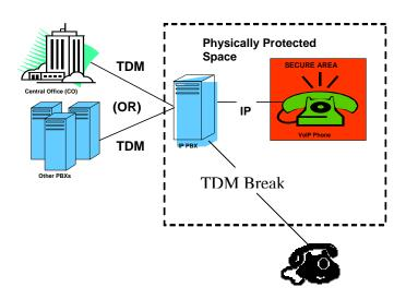
d. VoIP Trunk (Annex G). The trunk line is VoIP and the end telephonic device(s) and PBX is TDM as illustrated below. Either the Instrument or the TDM PBX provides security.
