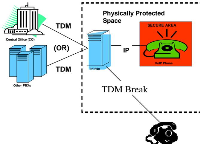
d. VoIP Trunk (Annex G). The trunk line is VoIP and the end telephonic device(s) and PBX is TDM as illustrated below. Either the Instrument or the TDM PBX provides security.
