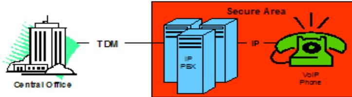
c. Hybrid VoIP (Annex F). A Hybrid VoIP, illustrated below, uses a mix of traditional TDM and VoIP technologies to complete the end-to-end call. However, unlike Isolated VoIP, the IP PBX is not required to be located in the secure area. Rather, it must be located in a Physically Protected Space (PPS). All signal lines must be protected to the same level as the PPS.
