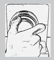
Dial RIGHT until your combination starts flashing. Your NEW combination will flash three times for the X-O7, but will only flash twice for the X-09.
